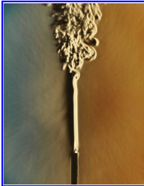
Figure 1.14: Imaging candle flow with Schlieren optics set up. Reproduced with permission from: https://commons.wikimedia.org/wiki/File:Laminar-turbulent_transition.jpg .
